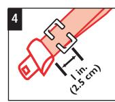
Position locking clip about 1 in. (2.5 cm) from vehicle belt's buckle plate.
